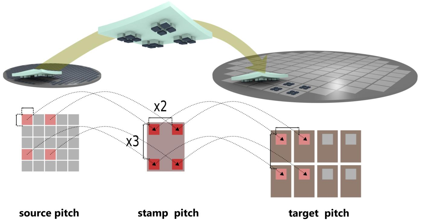
The target pitch has to be an integer multiple (1, 2, 3, ...) of the source pitch. The stamp pitch has to be an integer multiple of the source and the target pitch at the same time. In the example above the target pitch is two times the source pitch in horizontal und three times the source pitch in vertical direction. Stamp pitch and target pitch are equal.
