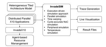
Fig. 1. Overview of the components and their connections of the InvadeSIM heterogeneous MPSoC simulator.
