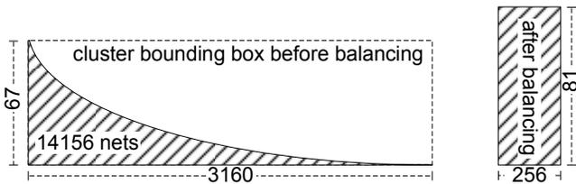
**Figure 5: Cluster balancing.** Example of balancing of one cluster in the JPEG decompressor design. Height represents the number of logic levels and width the number of gates. The cluster balancing algorithm takes clusters and reshapes them to a maximum 256 gates wide (limited by CUDA resources), while minimizing the height, which is the limiting factor in simulation latency.
