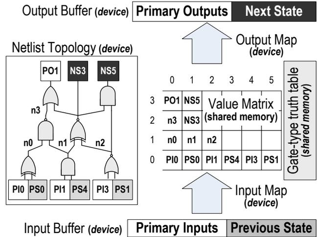
**Figure 3: GCS’s compiled-netlist data structures.** The picture shows the data structures required for the simulation of a small netlist. Thread blocks store and retrieve intermediate net values from the value matrix in the local shared memory. Note that there is a one-to-one correspondence between a row of intermediate values and a netlist’s logic level.
