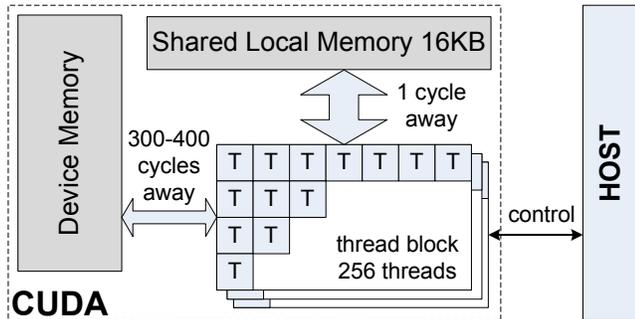
**Figure 1: The NVIDIA CUDA architecture** is organized as an array of multiprocessors. Each multiprocessor can execute a block of concurrent threads. A 16KB local shared memory block is available at each multiprocessor, which also has access to a larger, shared device memory.
