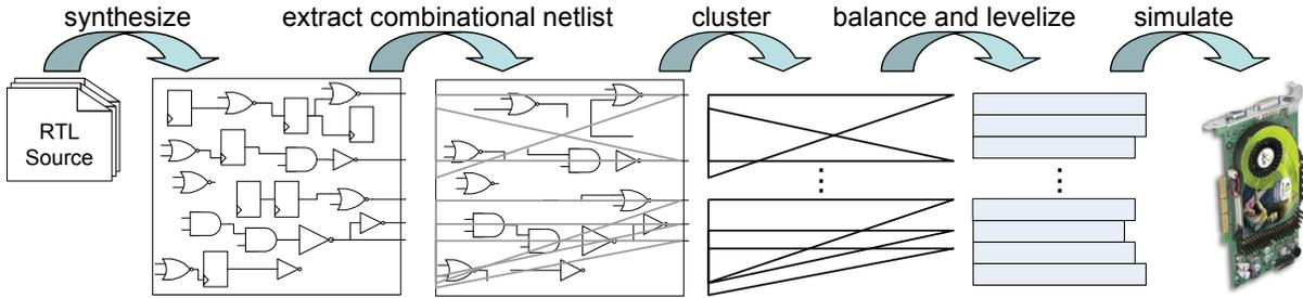
**Figure 2: The GCS compiler** considers a gate-level netlist or synthesizes a behavioral netlist. It then extracts the combinational logic block and partitions it into clusters, that is portions of the circuit that approximately fit within the resources of a single CUDA multiprocessor. The balancing step then optimizes each cluster to satisfy CUDA resource constraints. Finally, balanced clusters are transferred to the GP-GPU device and the simulation commences.
