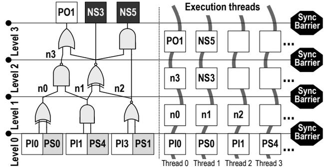
**Figure 7: GCS simulation on CUDA.** Simulation of the small netlist of Figure 3. Each thread is responsible for computing the output of one gate at a time, vertical wavy lines connect the set of value matrix slots for which a single thread is responsible at subsequent time intervals. Note also how each level is followed by a synchronization.
