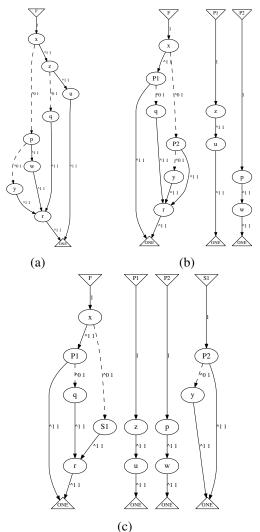
Fig. 2. Complex TED decomposition for  $F = x \cdot (z \cdot u + q \cdot r) + (p \cdot w + y) \cdot r$ : (a) Original TED; (b) Simplified TED after product term substitutions,  $P_1 = z \cdot u$  and  $P_2 = p \cdot w$ ; (c) Simplified TED after sum term substitution,  $S_1 = P_2 + y$ .
