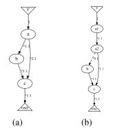
Fig. 1. TED representation for  $F = a^2c + a \cdot b \cdot c$ ; (a) Original, nonlinear TED; (b) Linearized TED representing factored form F = a(a+b)c.
