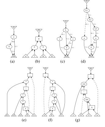
Fig. 3. Replacing constant multiplications by shift operations for expression  $F_0 = 7a + 6b$ : (a) Original TED; (b) Initial DFG; (c) TED after introducing a *shift* variable L; (d) Linearized TED; (e) DFG derived from the linearized TED; (f) DFG after combining variables  $L_i$  into L; (g) Final DFG after replacing multipliers by shifters.
