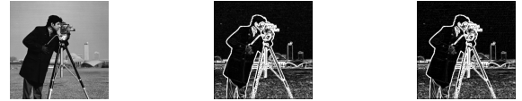
(a) Original image. (b) Exact. (c) Approximate. Fig. 6: Comparison of results from Sobel edge detectors using exact and approximate multipliers, respectively.
