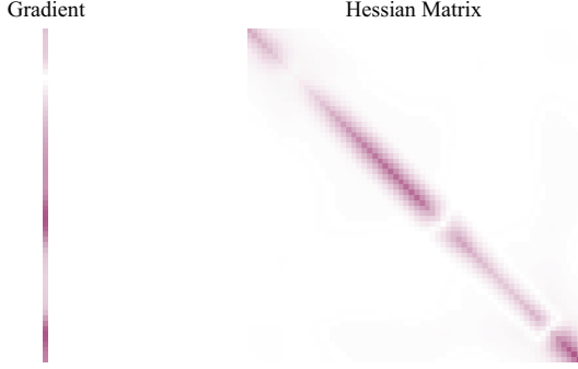
Fig. 3 Illustration of the gradient vector and Hessian matrix. The visualization highlights the diagonal dominance of the Hessian matrix in ILT, which inspires us to precondition the gradient using the inverse of Hessian matrix’s diagonal.
