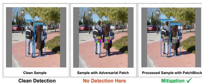
Fig. 1: PatchBlock in action: detecting and mitigating adversarial patches in real time. Example shows object detection using YOLOv4 [14] under AdvYOLO [15] attack on INRIA dataset [16].
