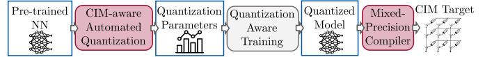
Fig. 1: Overview of the proposed framework. The main contributions are highlighted in red.
