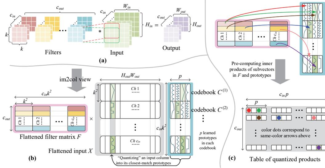
Fig. 1. CNN convolution in its (a) conceptual form; (b) equivalent matrix-matrix-multiply by flattening the filters and input features via `im2col`, with mapping of input data sub-columns onto the closest prototypes in different codebooks; (c) Precomputed inner products of  $F$ -subvectors and prototypes in a lookup table.
