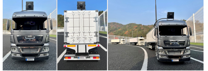
Fig. 1: Scale truck platooning testbed equipped with lidar, encoder, front- and rear-facing camera sensors.
