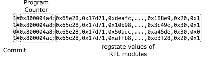
Fig. 2. Part of a microarchitectural trace generated by SIGFuzz. Each line in the microarchitectural trace represents a clock cycle during the test execution in the processor. The leftmost value in the trace is the commit signal, which indicates whether the program counter in the same row is committed in that clock cycle. The program counter located in the second column does not carry any meaning if the commit signal is zero. Each comma-separated value after the “:” sign represents the regstate value of an RTL module in the target processor.
