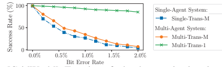
Fig. 4: [GridWorld] Transient fault characterization in GridWorld inference. Fault can impact only one action step (Multi-Trans-1) or whole sequential decision-making steps (Multi-Trans-M). Multi-agent system is more resilient to transient fault than single-agent system.
