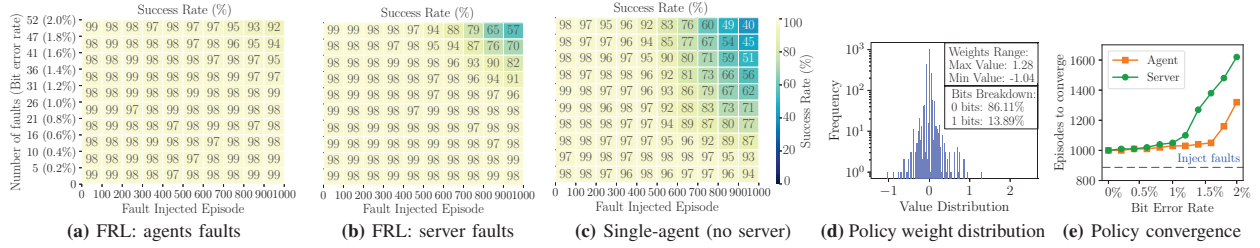
Fig. 3: [GridWorld] Transient fault characterization in GridWorld training, including (a, b) FRL and (c) single-agent systems. The fault impact is evaluated by average success rate of all agents within 1000 attempts for each scenario. FRL system is more vulnerable to server faults than agent fault. Single-agent system is more vulnerable to faults than multi-agent system. 0→1 flip has a higher impact than 1→0 flip, which can be explained by (d) policy weight distribution, where more 0 bits exist than 1 bits and policy has a narrow range. (e) shows episodes taken to converge after fault injected at the 900th episode. With training more episodes, system can recover from transient faults.
