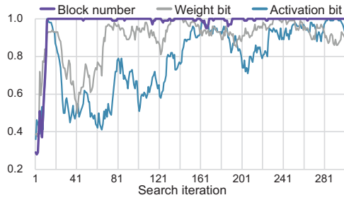
Fig. 3. Convergence of different design parameters. The y-axis indicates the proportion of the optimal candidates among all candidates (the closer to 1.0, the more convergent the parameter is).
