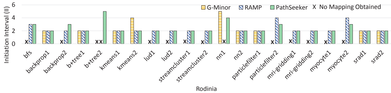
Fig. 3. Performance (II) comparison of PathSeeker with GraphMinor (G-Minor) and RAMP for application loops from Rodinia on a 4×4 CGRA.
