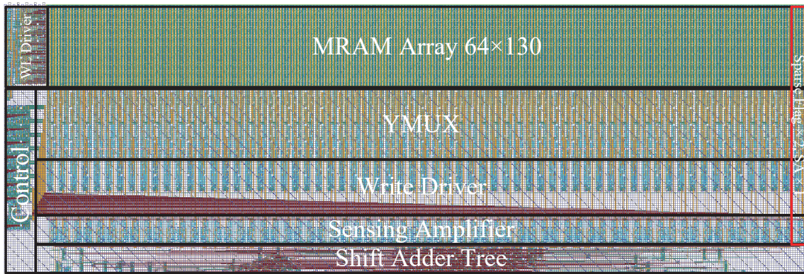
Fig. 5. Layout overview of main MRAM array (weight, 64 \times 65 \times 2 ), 2 sparse flags are implemented at the end of columns with 1 SA and shift adder tree is at bottom of the array.
