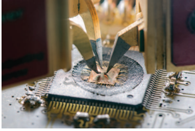
Fig. 6: Localized EM attack on a decapsulated IC
