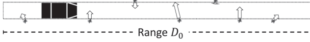
Fig. 4. N_j jaywalkers entering the path of the vehicle within the observed range D_o during the observation time T lead to an estimated flow density of \hat{j}_p = N_j D_o^{-1} T^{-1} .
