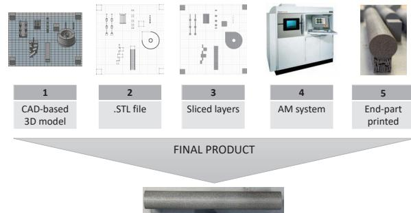
Fig. 1: AM process: main phases.
