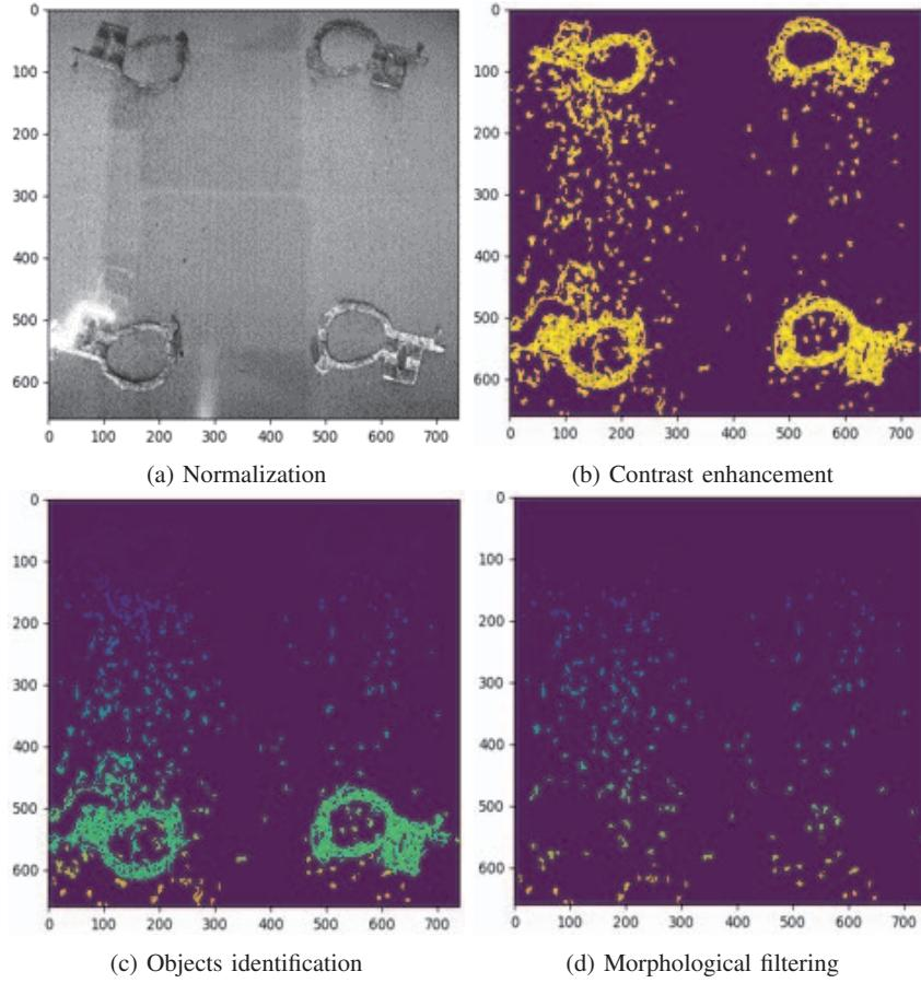
Fig. 4: Example of spattering defects detection pipeline.
