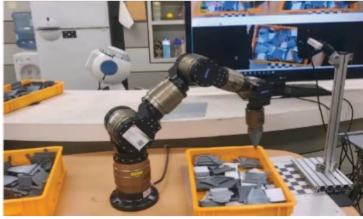
Fig. 23. A robotic bin picking scene that is set up to experimentally verify the application of the proposed CM-GAN to the 3D pose estimation of industrial parts in a bin
