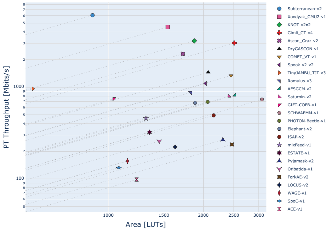
Fig. 1: Artix-7 Encryption PT Throughput for Long Messages vs LUTs
