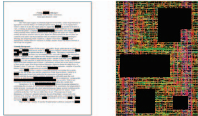
Fig. 1: Hardware redaction concept. Analogous to text document redaction, but in hardware, sections are removed and replaced with synthesizable eFPGA.
