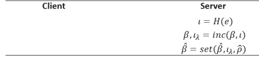
Fig. 4. Insertion. The server hashes the value e , increments the plaintext Bloom filter \beta at indices \iota , and set the encrypted Bloom filter \hat{\beta} at the indices \iota_\lambda where \beta became non-zero.
