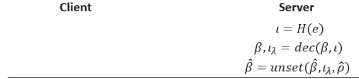
Fig. 5. Deletion. The server hashes the value e , decrements the plaintext Bloom filter \beta at indices \iota , and unset the encrypted Bloom filter \hat{\beta} at the indices \iota_\lambda where \beta became zero.
