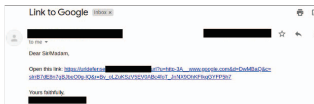
Fig. 7. URL denylist. Link to google.com is replaced by a link to a 3rd-party that checks if the link is in the denylist.
