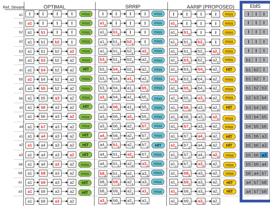
Fig. 1: Behaviour of OPT, AARIP and SRRIP using a Cf (A:{a1 ... a4}) and non-Cf application (B:{b1 ... b9}). The LLC reference stream is {a1, b1, b2, a2, b3, b4, a1, b5, a3, b6, a2, b7, a4, a1, a2, a3, b8, b9, a1, a3} a_{i_x} , b_{j_y} indicates the RRPV of cache blocks. SRRIP and AARIP here use M=2 to store the RRPV.
