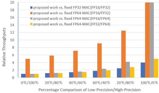
Fig. 8. Throughput comparison among fixed operations and the proposed multiple-precision dot product operations.
