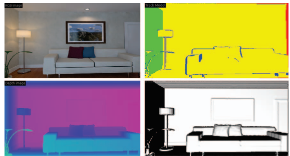
Fig. 2. The scene (top left), the input depth (RGB-D) frame (bot. left), the tracking output (top right), and the reconstructed 3D map (bot. right).
