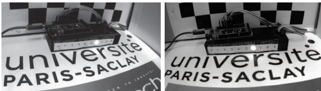
Fig. 3: Synchronous stereo acquisition of a LED chaser
