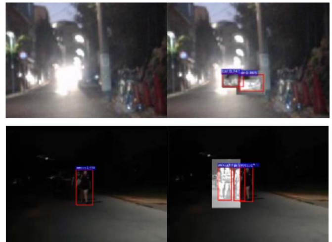
Fig. 5. Use cases for multiple visual modalities and application of modality control. Application of multi-modality control to Top: Light-cluttered scenes where a light sources completely saturates the visible spectrum reducing visibility of the scene and Bottom: Insufficient Illumination within the scene. Exposure time and gain has to be increased which leads to motion blur and noisy images. Multi-modality control allows us to switch the pixel modality while keeping track of the objects of interest.
