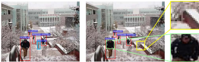
Fig. 4. Application of spatial resolution control to the problem of object detection. Note the elimination of the false positive highlighted in blue when feedback control is applied. In the right panel the insets show the difference between non-ROI and ROI regions. Yellow Inset: Non-ROI region, Green Inset: ROI Region
