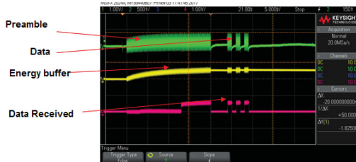
Fig. 9. Experimental evaluations were done with an oscilloscope monitoring the electrode output (first plot), the V_{supply} (second plot, yellow) and the data received by the microcontroller (last plot).
