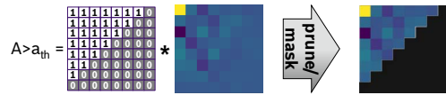
Fig. 3. Trained elements of the compression matrices below a threshold a_{th} are pruned whereas the remaining values are set to 1.
