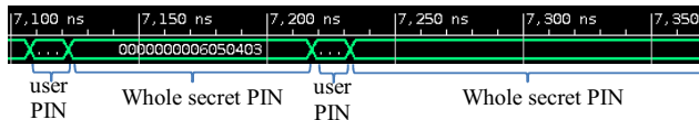
Figure 2: Chronogram showing that the whole secret PIN (3456) remains visible for long periods of time. It can be forwarded (with LSB at “11”).
