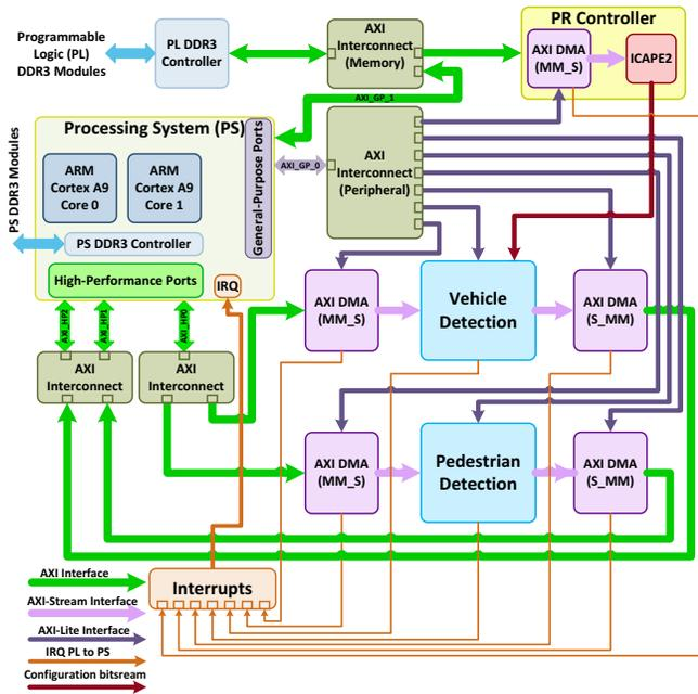
Fig. 6. Block diagram of implemented system and interfaces between the PS and PL components.
