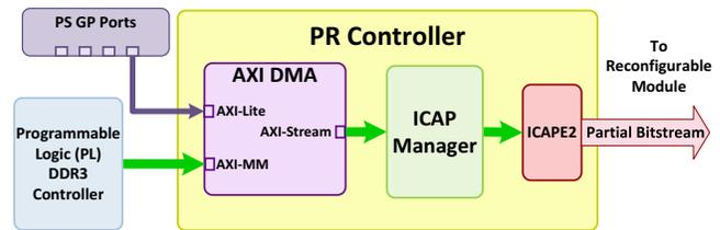
Fig. 7. Block diagram of partial reconfiguration (PR) controller.
