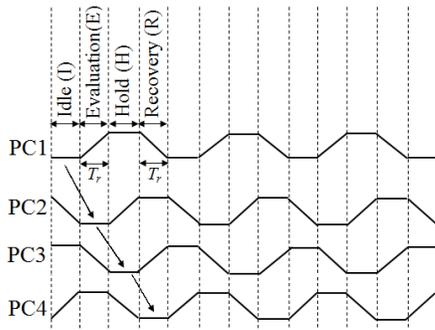
Fig. 2. 4-phase power-clocking scheme.
