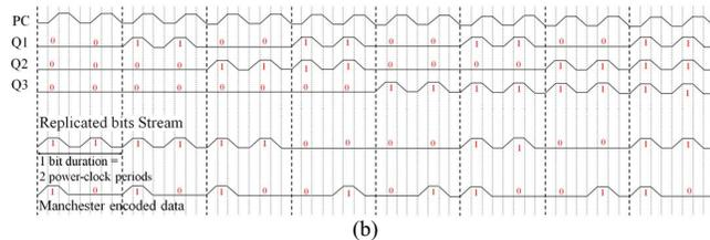
Fig. 5. Proposed Manchester encoding design output waveform.
