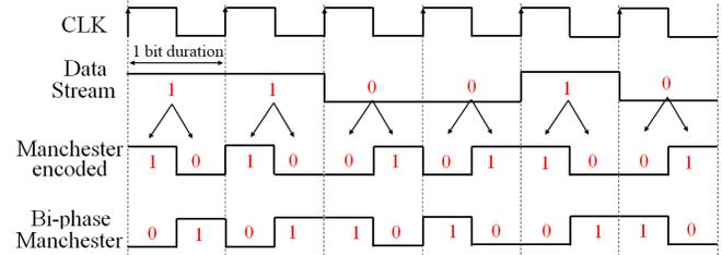
Fig. 3. Manchester encoding waveform
