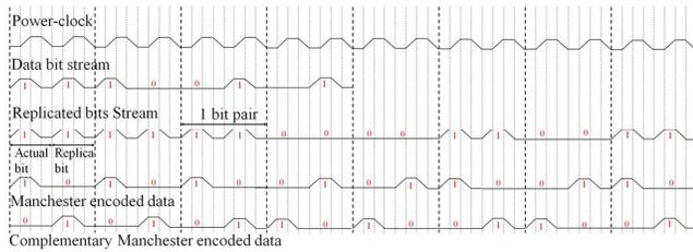
Fig. 4. Proposed Manchester encoding for adiabatic logic.
