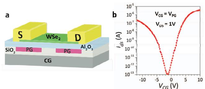
Figure 1. (a) 3D schematic of the fabricated devices. (b) Ambipolar transfer characteristics measured keeping  $V_{PG} = V_{CG}$ .
