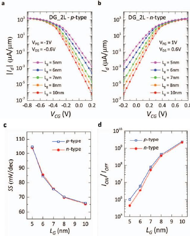
Figure 4. (a) Simulated transfer characteristics of *p*-type and (b) *n*-type FET. The gate length is varied from 10 nm down to 4 nm. (c) Sub-threshold slope, extracted from the simulated transfer characteristics for both *n*- and *p*-type behavior (d)  $I_{on}/I_{off}$  for both *p*- and *n*-type behavior. In both cases,  $I_{on}/I_{off} > 10^5$  is shown down to  $L_G = 5$  nm.
