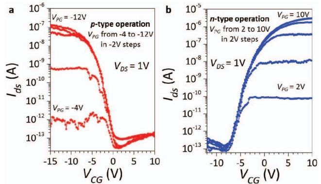
Figure 2. (a) Transfer characteristics of the device obtained for negative bias of the PG, showing *p*-type behavior and complete suppression of *n*-current. (b) Transfer characteristics of the device obtained for positive bias of the PG, showing *n*-type behavior and complete suppression of *p*-current.
