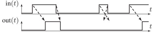
Fig. 2: Single-history channels allow to model pulse attenuation: The delay \delta(T) becomes smaller with smaller previous-output-to-input time T . Observe the cancellation of the second pulse due to non-FIFO-scheduled output transitions.
