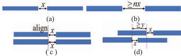
Fig. 2. Line-end spacing rules and wire patterns. (a) end-end spacing with normal x spacing; (b) end-end spacing with \geq nx spacing; (c) two line-end pairs with x spacing must be aligned; or (d) with the parity offset \geq y .
