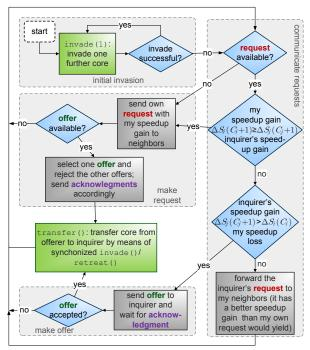
Fig. 3. Flowchart illustrating the communication scheme.
