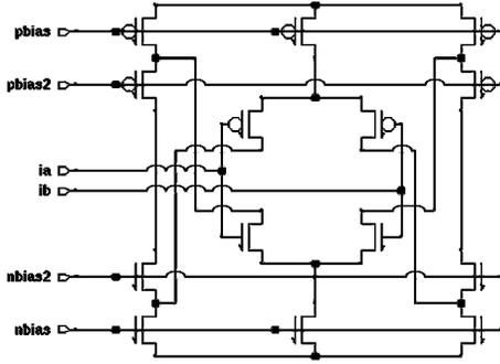
Figure 5. Differential amplifier with multiple bias points
