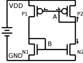
Figure 1. Simple circuit showing nodes (A, B, VDD, GND), devices (transistors p1, p2, n1, n2 and a voltage supply) and branch currents for node A
