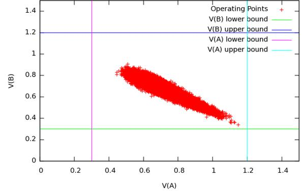
Figure 2. Map of verification results for circuit in Fig.1
