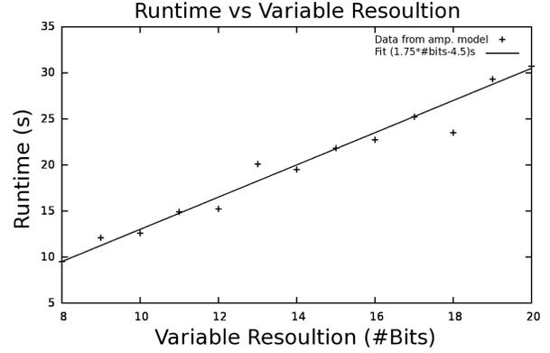
Figure 6. Time to solve for 4 bias voltages of circuit from Fig. 5 vs number of bits used to represent a voltage or current
