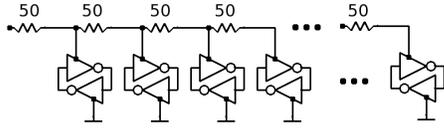
Figure 8. Schematic of SRAM array test. 10 SRAM cells used as part of this test
