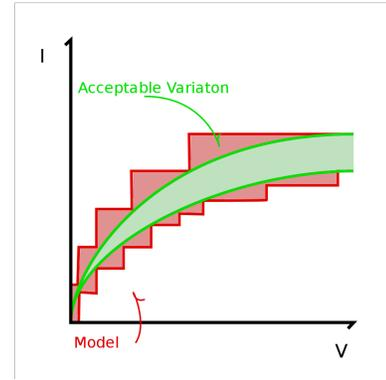
Figure 3. Transistor model, showing natural gutter of acceptable behavior and conservative discrete union of polytope model
