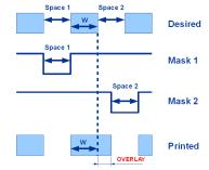
Figure 2. Example showing translation of overlay error into CD variation in negative-tone DP process.
