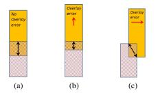
Figure 13. Example of a stitch in a vertical line (a), a possible failure with overlay error in Y direction that may occur after lineend pullback (b), and a possible failure with overlay error in X direction due to narrowing (c).
