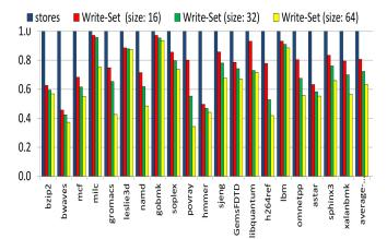
Fig. 3. Total entries in write-sets normalized according to the total number of store instructions in FaulTM.
