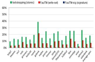
Fig. 4. The Error Detection Overhead of FaulTM vs Lockstepping in the Execution Time
