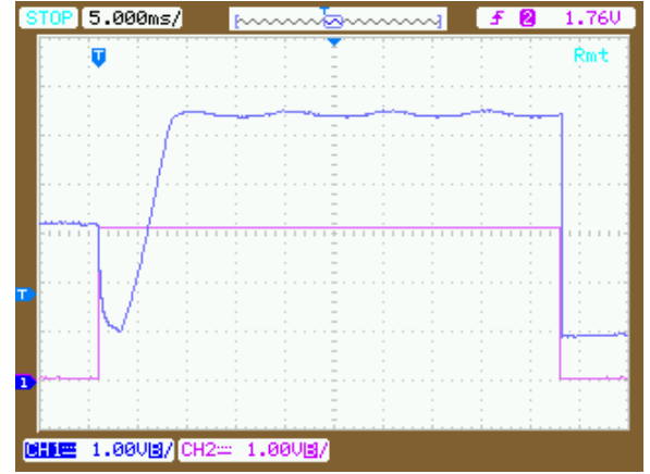
Fig. 4. Sampling operation taking place at 1000 lux. Shows the PULSE line which disconnects all loads from the solar cell and modifies the HELD\_SAMPLE line. A small ripple may be observed when the test is being carried out.
