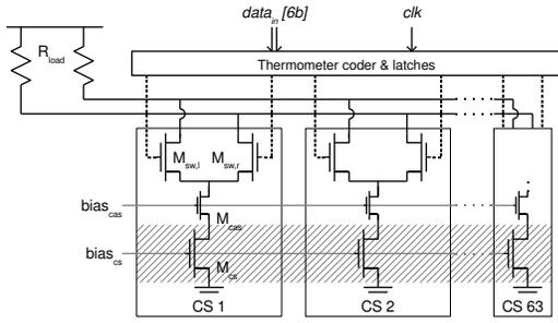
Fig. 4. Schematic of a 6-bit current-steering digital-to-analog converter. Reliability simulation is performed on the current-source transistors  $M_{CS}$ , shaded in gray, which are the accuracy-limiting transistors of the circuit.
