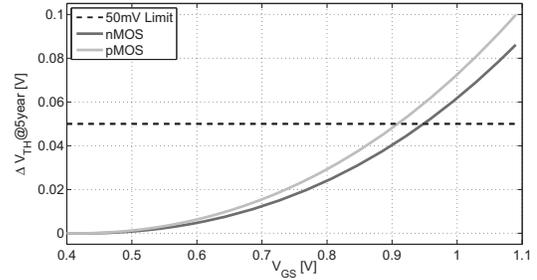
Fig. 3. Simulation of the threshold voltage shift after 5 years as a function of stress voltage for an nMOS and pMOS transistor in a predictive 32nm CMOS technology with  $V_{TH} = 0.38V$ . For a reliability margin of  $\Delta V_{TH} \leq 50mV@5year$  the maximum supply voltage is only 0.91V and is limited by NBTI.
