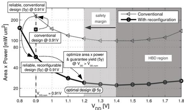
Fig. 6. Area-power product of the analog part of a standard and reconfigurable 6-bit DAC versus supply voltage. Optimal supply voltages can be found for both implementations. The reconfigurable design outperforms the conventional design both at the nominal supply voltage as well as at the optimized supply voltage.
