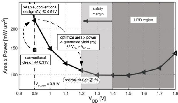
Fig. 5. Area-power product of the analog part of a 6-bit DAC versus supply voltage. Each design guarantees a 99.7% yield after 5 years. An optimum supply voltage can be found, making optimal use of the technology ( $V_{DD} > V_{DD,nom}$ ) and taking the expected degradation into account.
