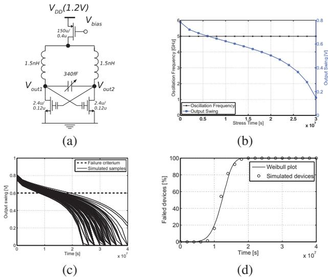
Fig. 2. Reliability simulation of an LC-VCO. LC-VCO (a). Nominal reliability simulation monitoring the oscillation frequency and the output swing (b). Dispersion of the output swing for 300 samples (c). CDF of the failure-time with a failure criterion set to an output swing less than 0.6V (d).
