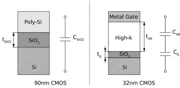
Fig. 1. Schematic representation of a traditional 90nm CMOS SiO<sub>2</sub>-based stack (on the left) and a 32nm CMOS high-k metal-gate HfO-based stack (on the right).
