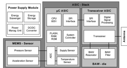
Fig. 5. Block diagram of the in-tire TPMS sensor node demonstrator
