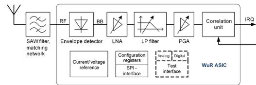
Fig. 9. Block diagram of wake-up receiver ASIC
