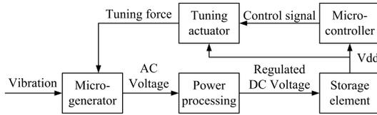
Fig. 1. Block diagram of a tunable energy harvesting system
