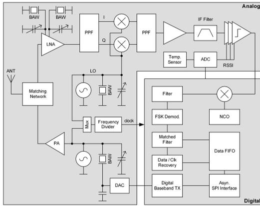
Fig. 6. Block diagram of the BAW transceiver
