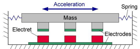
Fig. 8. Functional Principle of Vibration Scavenger
