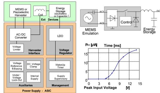
Fig. 7. Block Diagram of the Vibration Scavenger based Power Supply Subsystem
