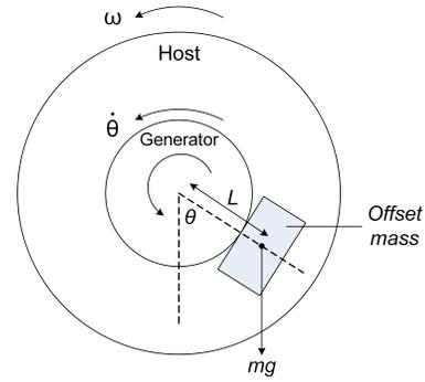
Fig. 2. Diagram of a rotational energy harvester [14] (reproduced with permission)
