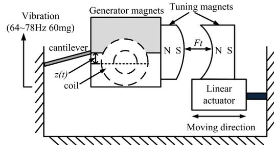
Fig. 3. Tunable electromagnetic microgenerator [16]
