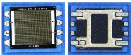
**Fig. 2** – Optical microscopy image of a large area SiPM in a suitable SMD package in Top (left) and Bottom (right) view.
