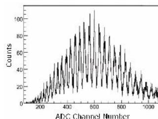
**Fig. 3** – Typical charge spectrum obtained in low intensity illumination regime on a large area SiPM. Each peak corresponds to an activated microcell (i.e. a detected photon) [3].
