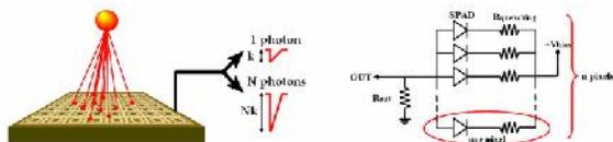
**Fig. 1** Left - Scheme of principle of a silicon photomultiplier (SiPM) based on an array of SPAD sensors with passive common readout; Right - Electrical scheme of the SiPM, biasing circuit and output signal extraction.
