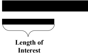
Fig. 6. For two parallel lines, the length we are interested in is the length for which the two lines run side by side.
