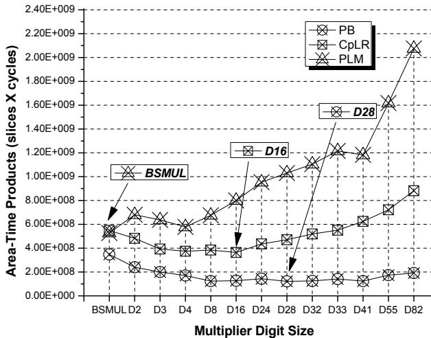
Fig. 8. Comparison of time-area products for each configuration of coprocessors
