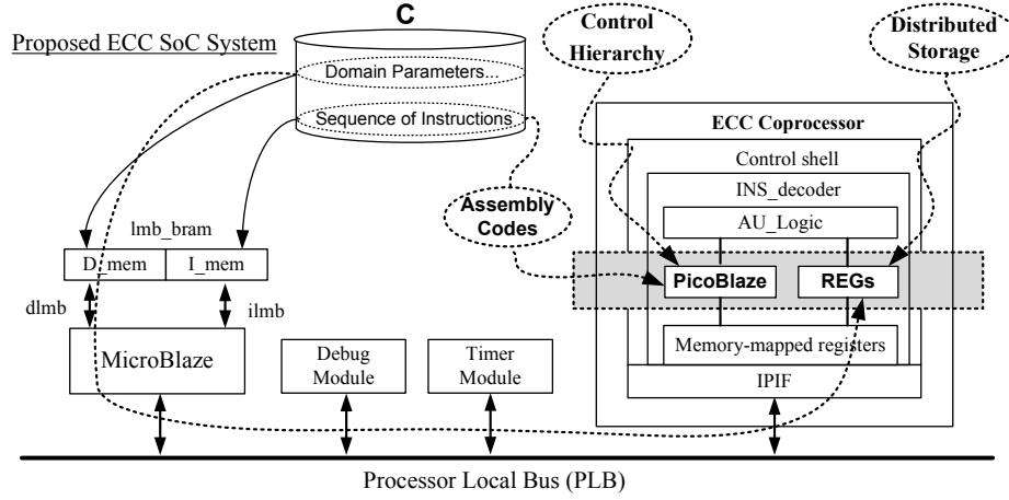
Fig. 5. Block diagram of proposed ECC SoC system
