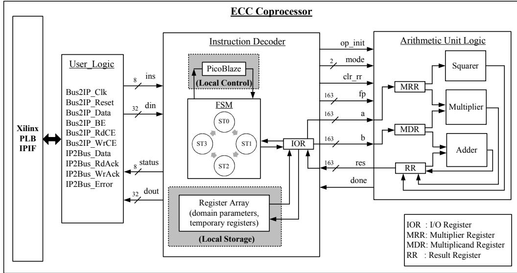
Fig. 6. The structure of proposed ECC coprocessor
