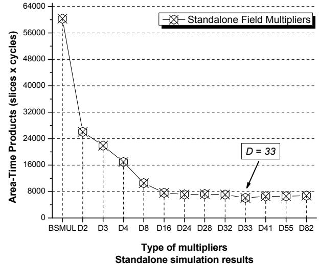
Fig. 2. Area-Time products of the different multiplier implementations
