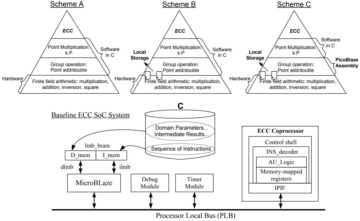
Fig. 3. ECC system schemes and block diagram of baseline ECC SoC system
