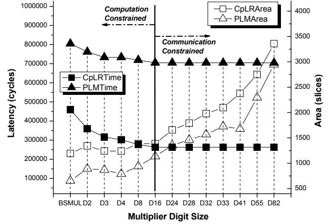
Fig. 4. Time to complete one multiplication and area for each type of coprocessors
