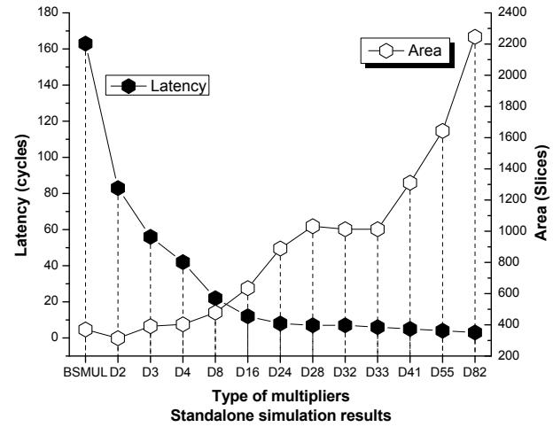
Fig. 1. Time to complete one multiplication and area for each type of multipliers
