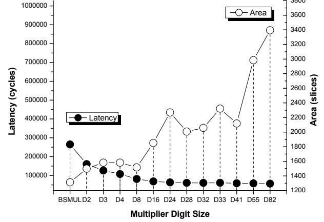
Fig. 7. Time to complete one multiplication and area for each configuration of coprocessors
