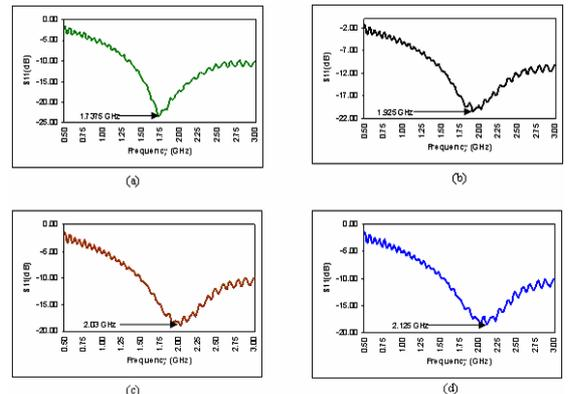
Fig. 6 Four  $S_{11}$  curves for the adaptive LNA
