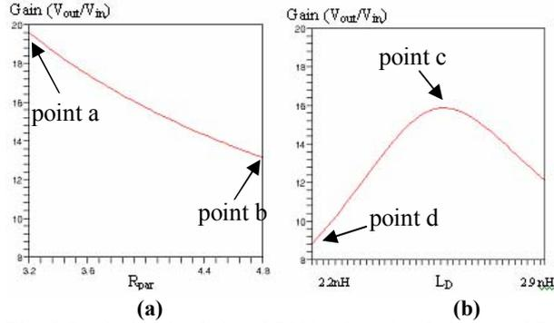
**Fig. 3 Deviation in Gain of LNA when (a) Q-factor of  $L_D$  changes by 25% (due to soft-fault or variation) and (b) when  $L_D$  varies by 30%**
