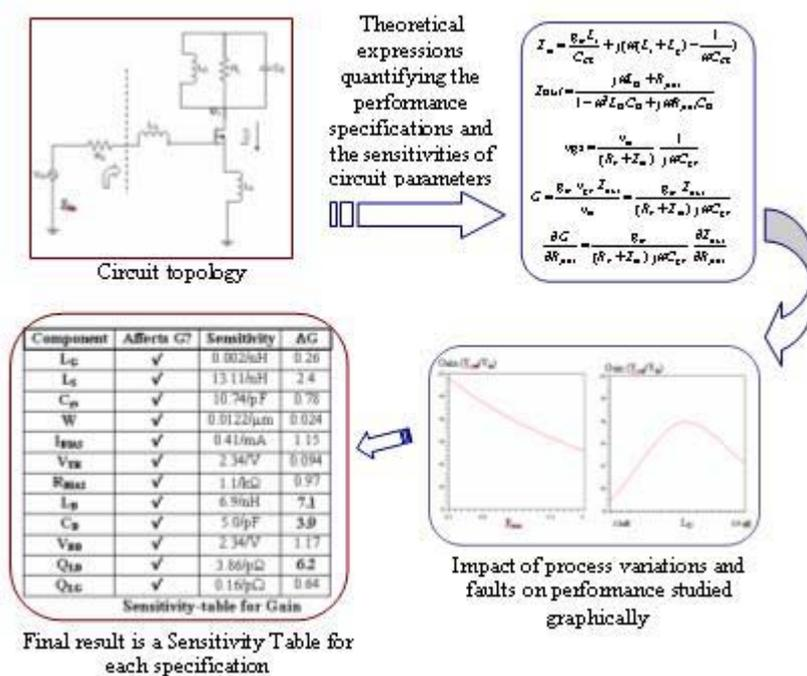
Fig. 1. The Sensitivity Analysis Flow
