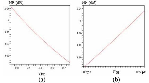
Fig. 5 Impact on NF when (a)  $V_{DD}$  is varied by +/-10% and (b)  $C_{GS}$  is varied by 10%
