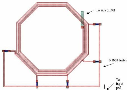
Fig. 7 The tapped gate coil
