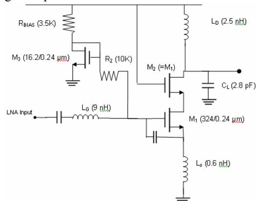
Fig. 2 Cascode LNA used in this work
