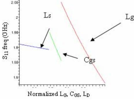
Fig. 4 Variation in  $S_{11}$  frequency (in GHz) for  $L_S$ ,  $L_G$  and  $C_{GS}$  tolerances
