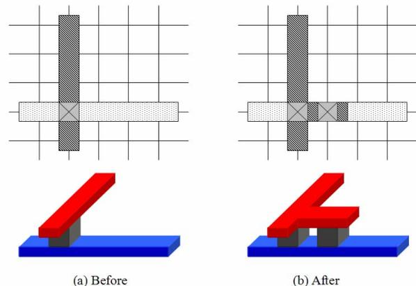
Fig.1: Redundant via insertion.
