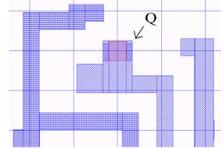
**Fig. 7: Unable to place double vias on pin Q.**
