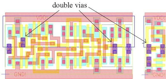
**Fig. 6: Double vias on pins of DFF (left) and NAND2**
