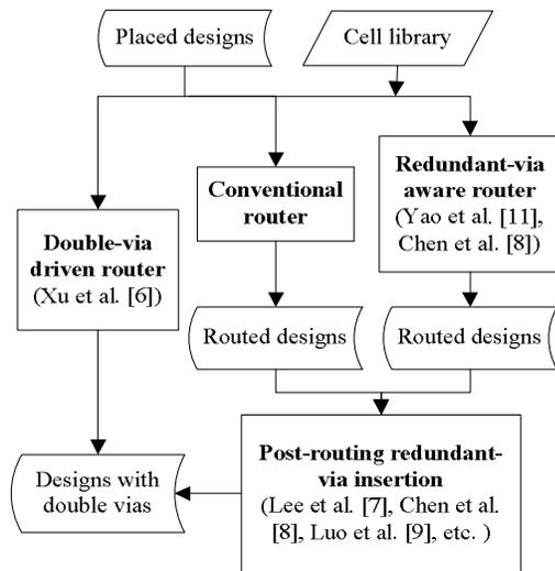
**Fig. 2: Approaches to double-via placement.**
