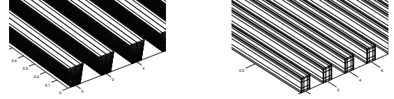
Fig. 5. Structural view of an array of 8 conductors with (a). trapezoidal cross-sections and (b). rectangular cross-sections.
