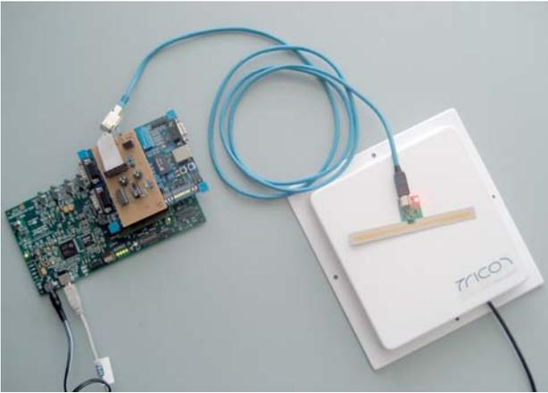
**Figure 8. Development hardware in UHF RFID environment**
