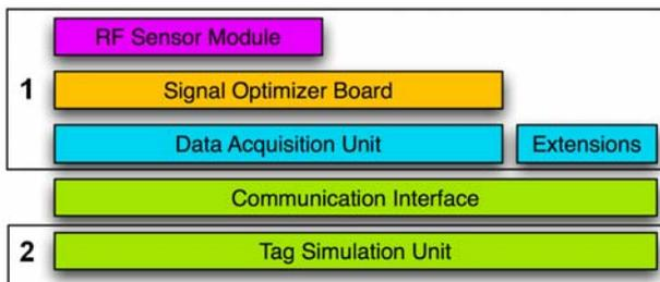
Figure 3. Hardware module stack of the simulation platform
