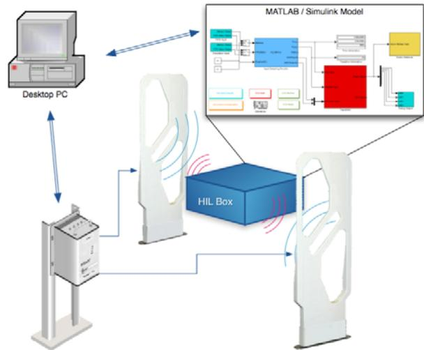
Figure 2. Proposed solution for UHF RFID system verification
