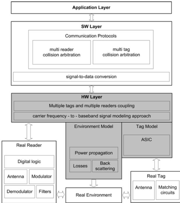
Figure 1. Framework for UHF RFID simulation
