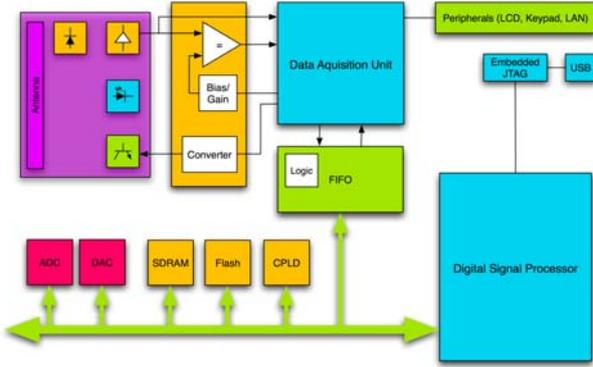
**Figure 6. Block model of the HW simulation platform**
