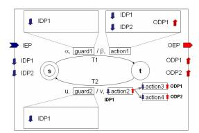
Figure 3. A simple EFSM component model.
