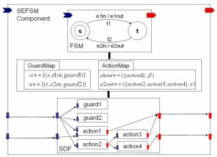
Figure 4. A compositional structure of the EFSM component originally shown in Figure 3.
